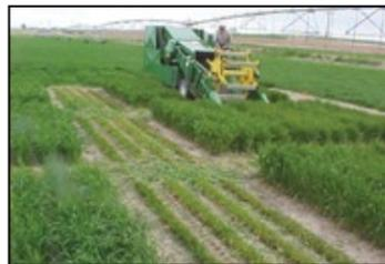
Harvesting small grains forage using a plot harvester.
