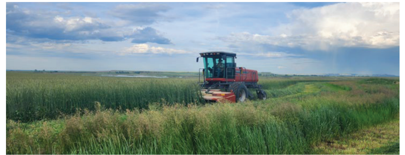
Swather cuts hay for drying prior to baling. Photo by James Sedman.
